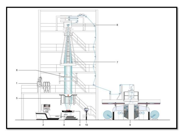
Diagram of the extrusion process
