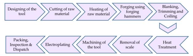
**A. Designing of the tool:** A designing software like Solidcam will be used for designing of the tool as per the client requirements. Designing operations will
