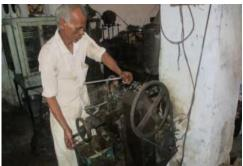
Conventional drilling machine in a hand tool unit
